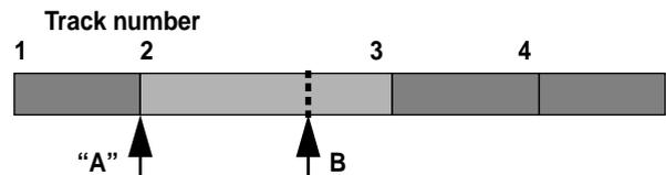
This provides a convenient way in which data can be erased from the start of a track only.
